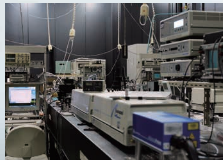
Titanium:Sapphire laser system for the femtosecond pump-probe spectrometer (Condensed Matter Dynamics Group).
