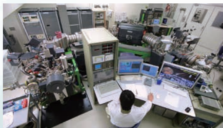
Isotope microscope used for the survey of the isotopic composition of asteroidal materials.
