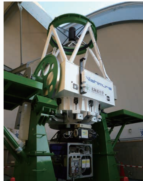
Pirka telescope with an effective aperture of 1.6 m for planetary and astronomical observations.
