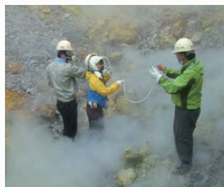
Picture of the field measurement showing the sampling of the hot volcanic gas.
