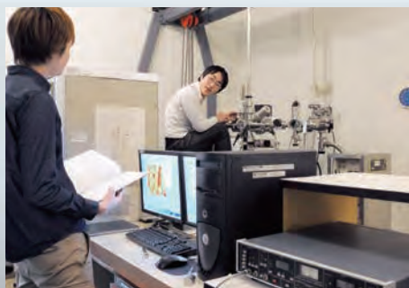
Experiments by using of low-temperature high-vacuum scanning tunneling microscope (STM) (Electric Properties of Solids Group).
